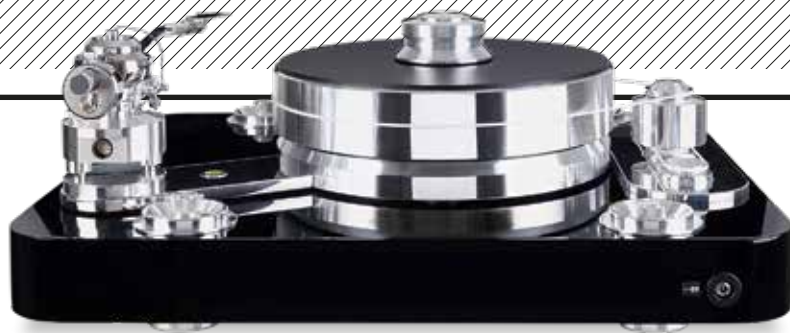
ABOVE: The rear of the plinth carries the 15V PSU input [right] while the delicate tonearm wires exit the top of the bearing and are terminated in a secure 5-pin socket at the base of the arm [left]. This is a standard fitting supporting aftermarket cables
