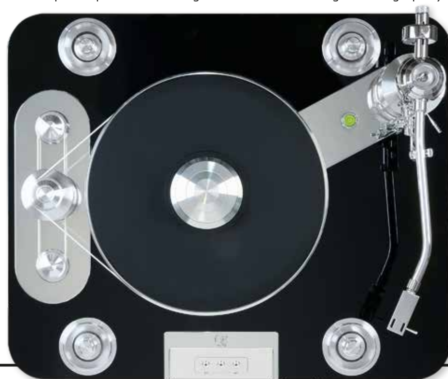
RIGHT: The alloy 'islands' for the dual AC motor/flywheel drive [left] and tonearm outrigger [right] are isolated from the MDF plinth with TPE damping. The inset spirit level [green, top right] is a thoughtful addition
